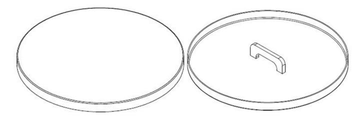
The 22" cover is shoebox style and will fit loosely on top of tanks to keep dust, dirt and debris from entering the tank and contaminating product. The floating cover sits in inside the tank and floats up and down on the liquid to help prevent evaporation of product. The floating cover has a handle in center.
